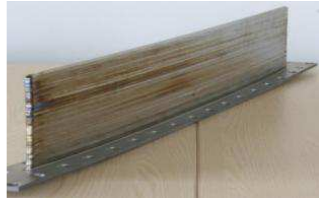
Ti walls 1000x200x4 mm 3 – mechanical test pieces – O 2 ~1500 ppm
