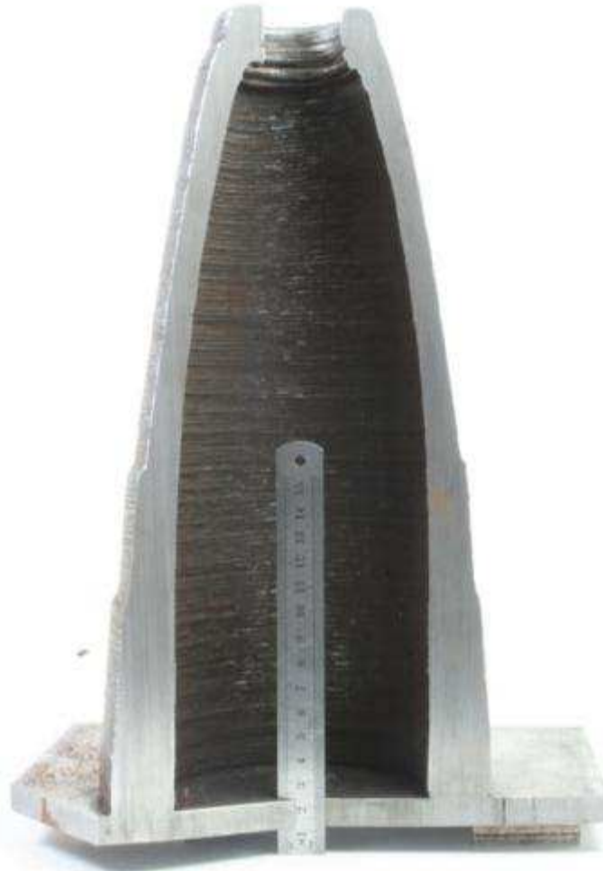
Variable wall thickness ogive with overhang for threaded section
