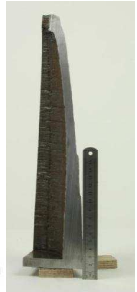
Variable wall thickness ogive with overhang for threaded section
